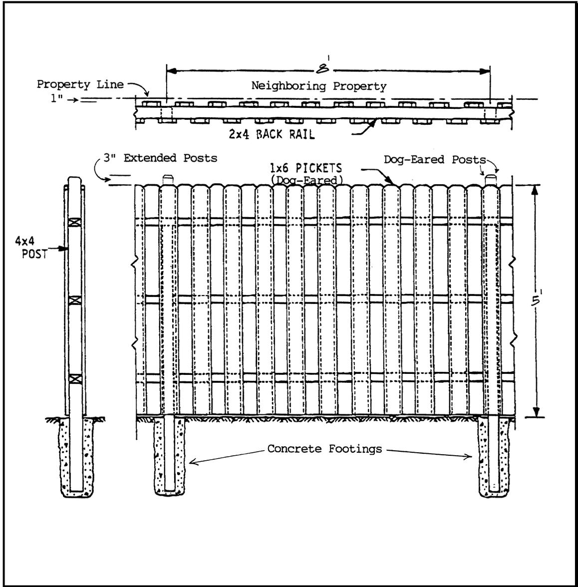
Figure 3.03-1: Drawing details for a standard fence addition.
